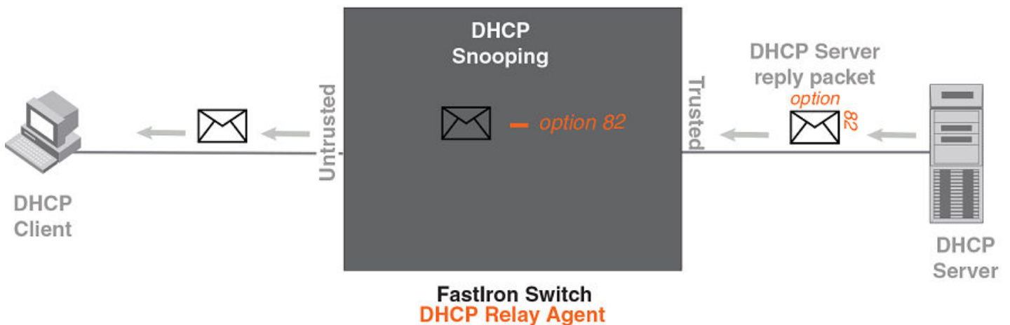
FIGURE 11 DHCP Option 82 Attributes Removed from the DHCP Packet
